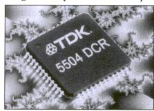
frequency range of 950 to 2150 MHz. The device accepts an input signal in this frequency range and down-converts directly to baseband. The local oscillator signal is generated by a completely integrated phase-lock loop that is fully programmable through a standard serial port interface.
