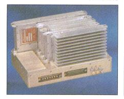
direct digital synthesis with microwave mix/divide circuits to accomplish performance specifications, such as a frequency resolution of 0.7 Hz, a switching speed of 150 ns and high spectral purity. Standard models operate from 1.6 to 2.8 GHz. The internal oscillator is free running or phase locks to an external 10 MHz reference.
