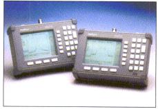
powered by a lightweight NiMH battery. The instrument covers  $100~\mathrm{kHz}$  to  $3~\mathrm{GHz}$ , which includes a wide range of today's communications systems. It has  $65~\mathrm{dB}$  dynamic range,  $\pm 1.5~\mathrm{dB}$  amplitude accuracy, a full-span noise floor of  $-97~\mathrm{dBm}$  and minimum resolution bandwidth of  $10~\mathrm{kHz}$ . The MS2711A is priced at \$7,000 with four to six weeks delivery.
