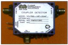
tor with output optimized to operate over 2.4 to 2.5 GHz with a VSWR of 1.5 to 1. This unit has SMA connectors on the RF and TTL output and solder pins for the DC power and control.
