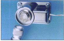
this panel receptacle avoids the cumbersome use of safety covers and other devices to achieve its safety goal. It operates on 4 to 24 VDC and is constructed with either gold or silver center conductors, beryllium-copper contacts, Teflon® insulators, and brass bodies. The 7-167 interlock switch panel receptacle is priced at approximately \$89 each, depending on quantity.
