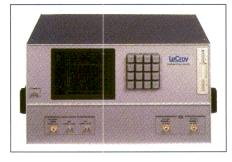
60 GHz input channels, a 6.24 to 200 MHz TTL output, 6.25 MHz to 1.6 GHz ECL output and an impulse output with frequency content from 6.25 MHz to 60 GHz. There are also GPIB, VGA and Centronics ports, plus connections for 10 MHz reference in/out. Applications include broadband TDR measurements, phase and group delay measurement and frequency domain transmission and return loss measurements in microwave radio and many optical communications systems.
